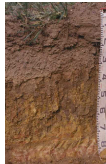
Variant with shallower profile and greater (80%) and coarser (10-40 mm) gravel content
